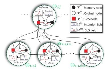
Fig. 1: Illustration of the structure of a single elementary behavior (EB) and the inter- and intra-layer coupling for the hierarchical organization of sequences.
