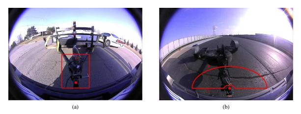
Fig. 2: 2a The surrounding of the hitch that is taken into account for detecting the presence of a trailer. 2b The definition of the polar coordinate system to transform the area around the hitch for later symmetry analysis.
